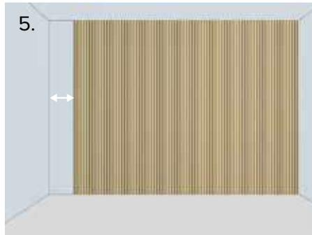
5. Install in turn. Measure the remaining width
