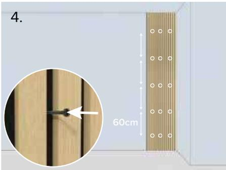
4. Place the acoustic panel on the wall and nail it.
