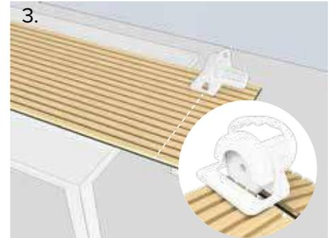
3. Cut the acoustic panel according to the height of the wall.
