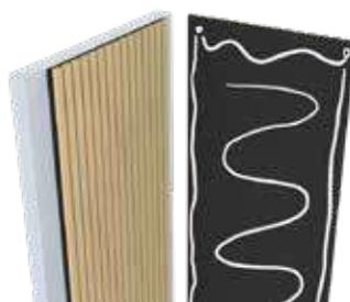
**C** Install fibreglass wool or rock wool between the battens.
