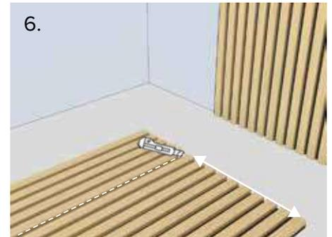
6. Cut the acoustic panel into the remaining width.
