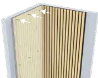
**B** Attach acoustic panels to the wall with nail-free glue.
