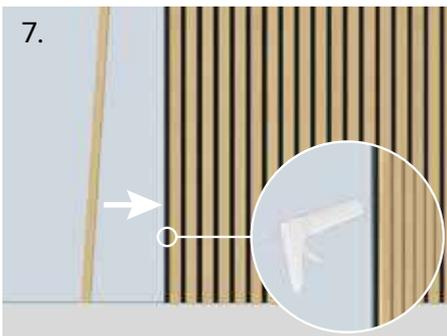
7. Use an edge strip at the edge. Glue the edge of the acoustic panel and stick the edge strip firmly at the gluing place.
