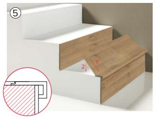
Place the floor plank anchoring it with the Loc system.
